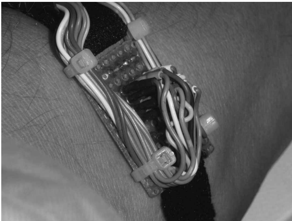
Figure 6. Measurement device for the determination of the electric potential difference. Four times four electrodes serve as sensors and are placed in a distance of 2.4 mm from each other onto the skin surface.
